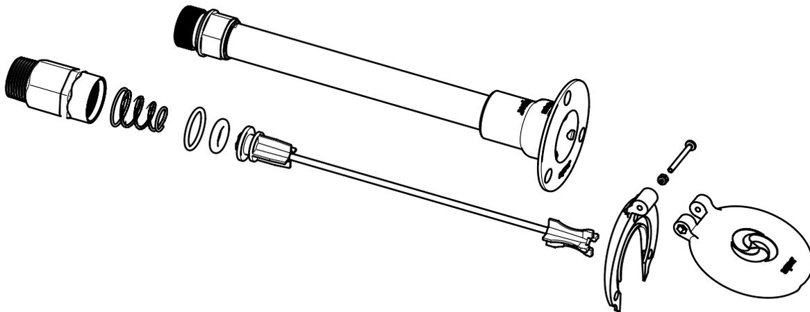
A simple valve design ensures maximum reliability. There is only one moving part, the stainless steel inner rod that operates the rear closure. A spring holds the valve shut in the event of loss of pressure.
