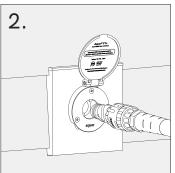
To connect, align the 3 grooves on the connector with the nibs on the hydrant. Gently push in, then twist clockwise.
