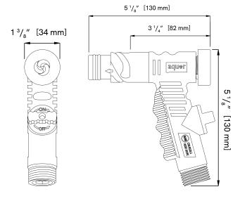
The Vacuum Breaker Connector provides backflow prevention. Can be used with any of our hydrants or outlets. The angled handle provides extra leverage for ease of use. Integrated ball valve for flow control. Use with or without a garden hose.
