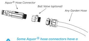
Some Aquor<sup>®</sup> hose connectors have a one-way check valve to prevent water from spraying when you disconnect.
