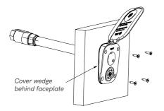
Tip: Drilling into brick or stone? Consider using specialized fasteners and/or anchors. We also manufacture optional stainless steel mounting plates to space the mounting holes out further if needed.
