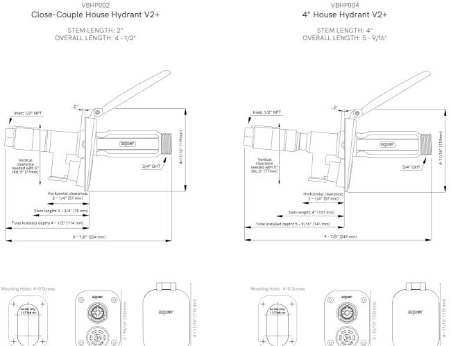
Using a 1.5" hole saw is suggested. You may also cut a rectangular hole.
