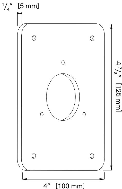
For retrofits. Great for brick and stucco and many siding types. Plate extends the mounting screws further from the entry hole—perfect for crumbling masonry or covering larger entry holes. Hydrant attaches to the mounting plate with included machine screws.
