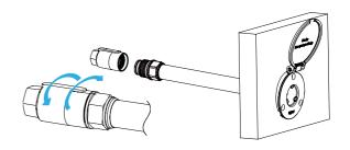
With the appropriate fitting installed, re-attach the inlet to the hydrant body.
