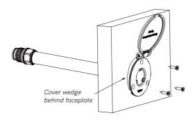
Tip: Drilling into brick or stone? Consider using specialized fasteners and/or anchors. We also manufacture optional stainless steel mounting plates to space the mounting holes out further if needed.
