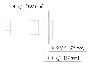
Flush-mounted stainless steel hydrant with hose connector. A reliable, leak-proof water outlet that can be used anywhere water access is needed, on land or sea. Ideal for marine vessels, campers, RVs, overland vehicles, storage tanks, DIY applications, and much more. Can be mounted horizontally or vertically.
