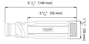
Attach to any garden hose and leave attached for easy water access. Internal one-way valve eliminates sprays or backflow. Connect under full water pressure and easily swap between hoses and nozzles in seconds with a simple push and twist.
