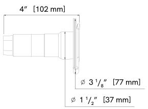
Flush-mounted stainless steel hydrant with hose connector. A reliable, leak-proof water outlet that can be used anywhere water access is needed, on land or sea. Designed for pressurized water sources attached via hose. Installs vertically or horizontally. Can be used for incoming or outgoing water flow. Rubber EPDM plug cover fits snugly into outlet, sealing out any dirt or debris when not in use.
