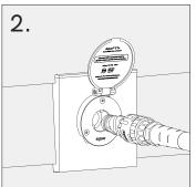
To connect, align the 3 grooves on the connector with the nibs on the hydrant. Gently push in, then twist clockwise.
