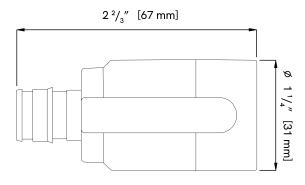
This inlet replaces the default hydrant inlet with a 1/2'' PEX F1960 connection. Quickly and reliably connect your Aquor hydrant to 1/2'' PEX tubing with a cold-expansion connection.
