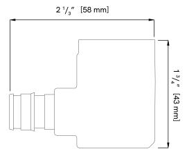
This inlet replaces the default hydrant inlet with a 1/2'' PEX F1960 connection. Quickly and reliably connect your Aquor hydrant to 1/2'' PEX tubing with a cold-expansion connection. The elbow inlet shortens the overall length of the hydrant by 1/2''.
