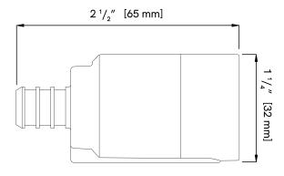
This inlet replaces the default hydrant 1/2" NPT inlet. Quickly and reliably connect your Aquor hydrant to 1/2" PEX tubing with a crimp connection.
